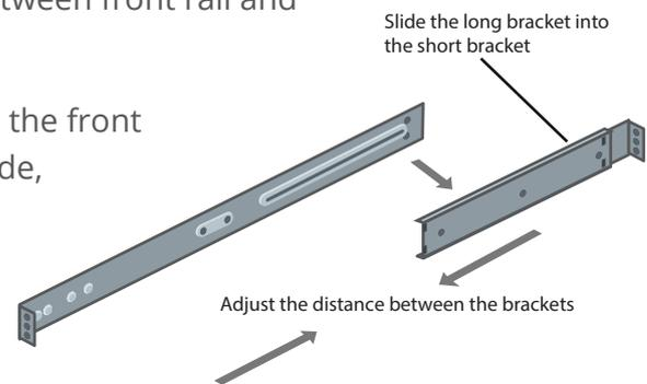
3. Adjust the short and long brackets to the proper distance so that the chassis can perfectly fit into the rack.
