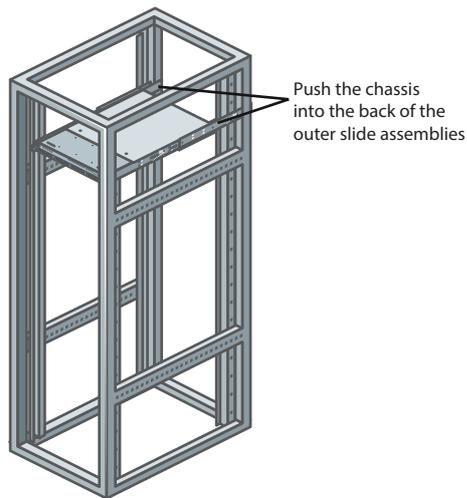
2. Push the chassis till the back of the outer slide assemblies as shown below.
