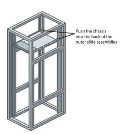
2 Push the chassis till the back of the outer slide assemblies as shown below.
