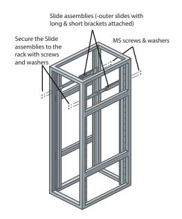
Depending on your rack structure, short brackets might not be required to attach to the outer slide.
