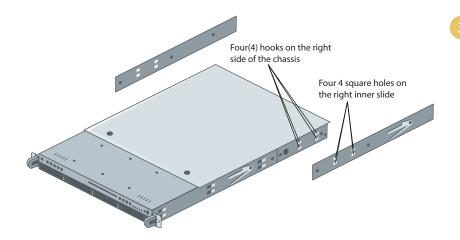
Attach the slide to the chassis with two M4 flat head screws and repeat the steps from 1 to 3 to install the left inner slide to the left side of the chassis.
