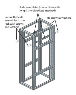
**Note:** Depending on your rack structure, short brackets might not be required to attach to the outer slide.
