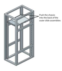
2. Push the chassis till the back of the outer slide assemblies as shown below.
